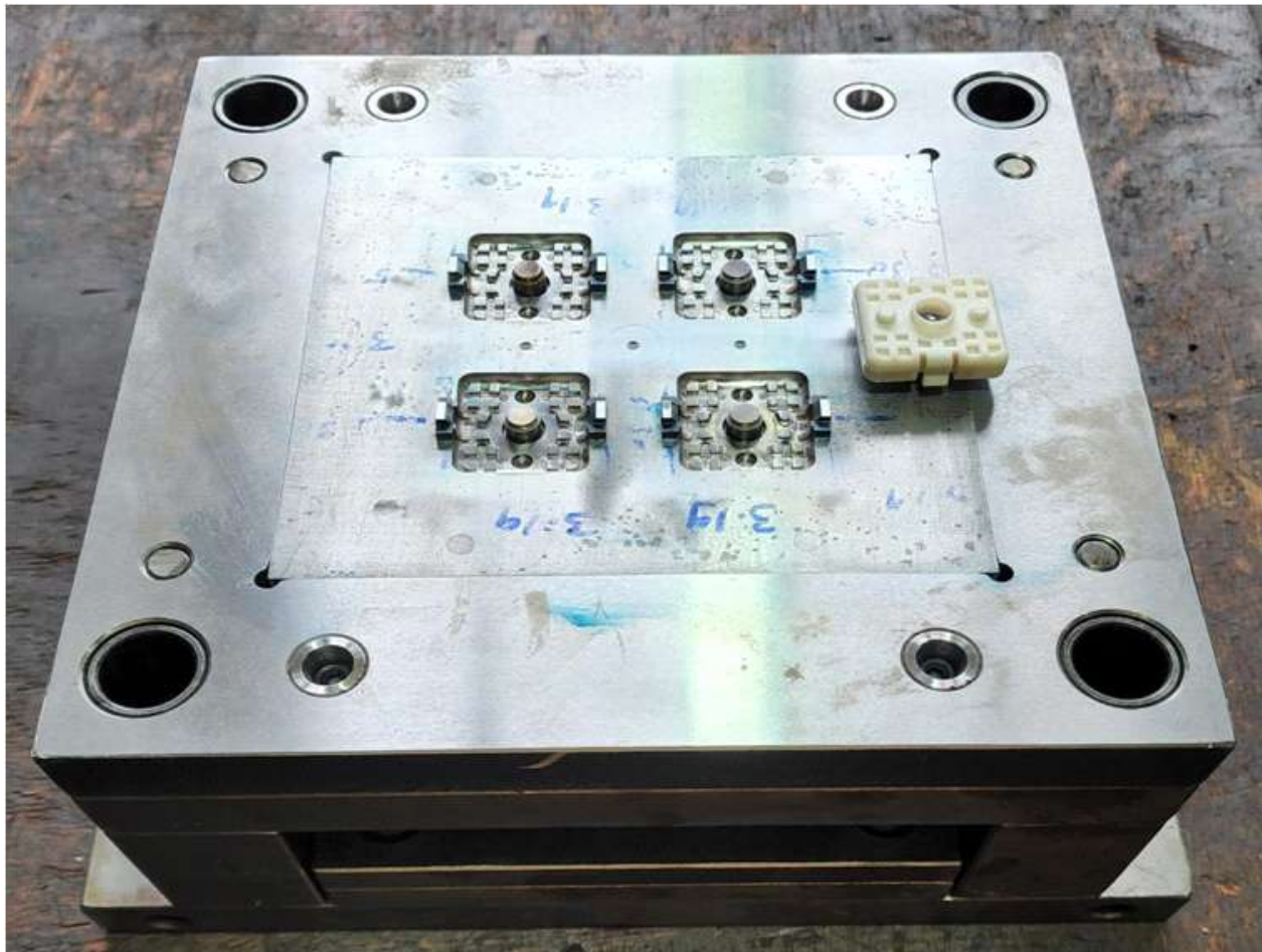
4 CAVITY ISOLATION ELECTRICAL PART - M8 MOLD
